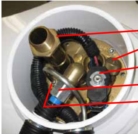
Figure 10. LPI tank valves. The valves are located under the access plate. See Figure 11.
