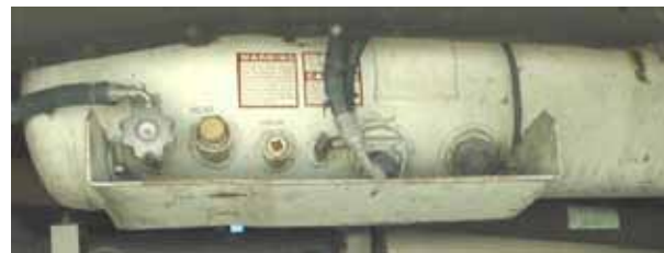
Figure 30. Tank located inside the frame rail, opposite the exhaust catalyst
