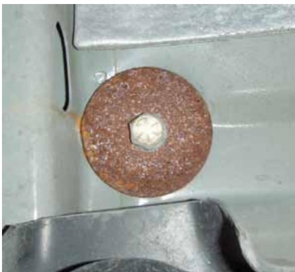
Figure 19. Load-spreading washer located under vehicle bed
