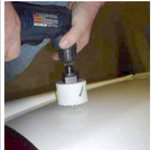
Figure 44. Drilling body panel for pass-through of hoses or fittings
