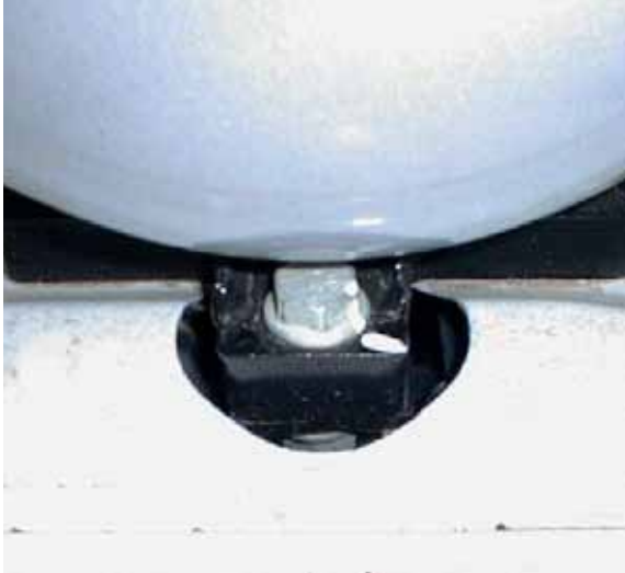
Figure 21. OEM tank installation showing through-bed mounts
