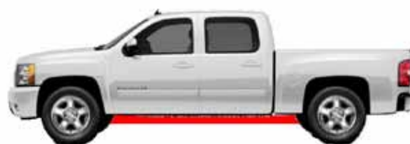
Figure 26. No tank mounting below the shaded area
