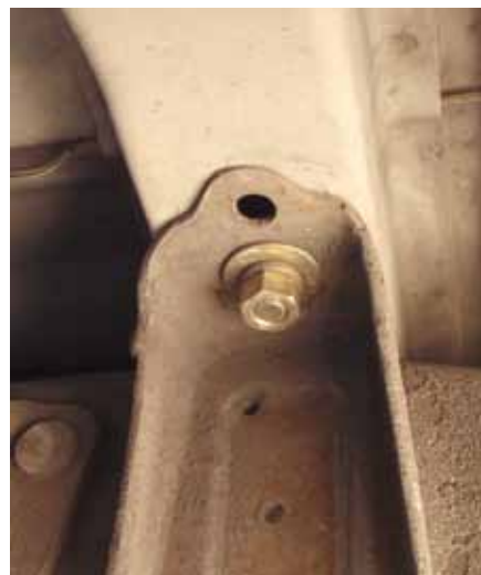
Figure 18. Bed-mount installation that also serves as a tank mount
