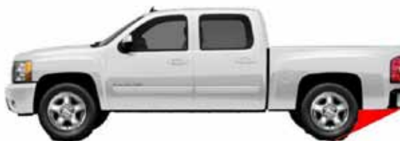
Figure 27. No tank mounting below the shaded area
