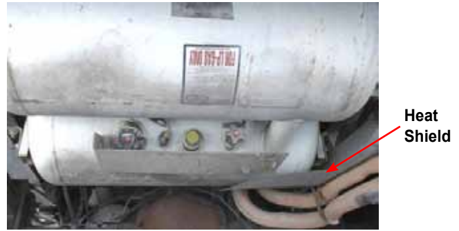
Figure 28. Manifold tank installed behind the axle in the original tank location
