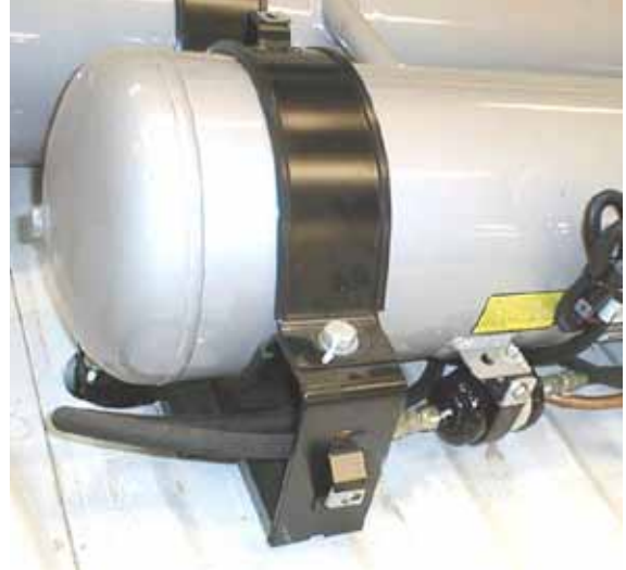
Figure 22. OEM tank installation showing through-bed mounts
