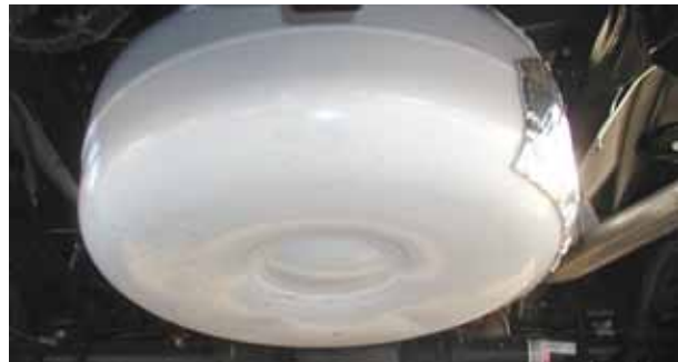
Figure 31. Toroidal tank installed in spare tire location behind rear axle
