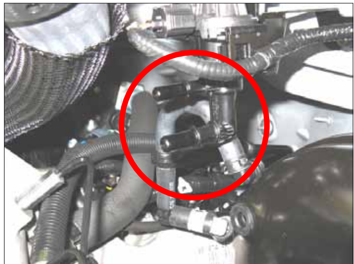
Figure 47. Disconnected evaporative canister purge valve
