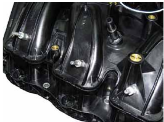
Figure 28. Injector nozzles installed in drilled and tapped locations
