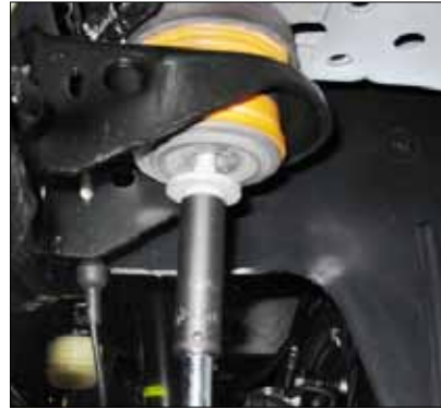
Figure 50. Loosening body-to-chassis mounting bolts with hand tools
