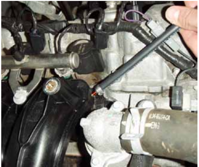
Figure 29. Nozzle installation using hex wrench inserted through hose
