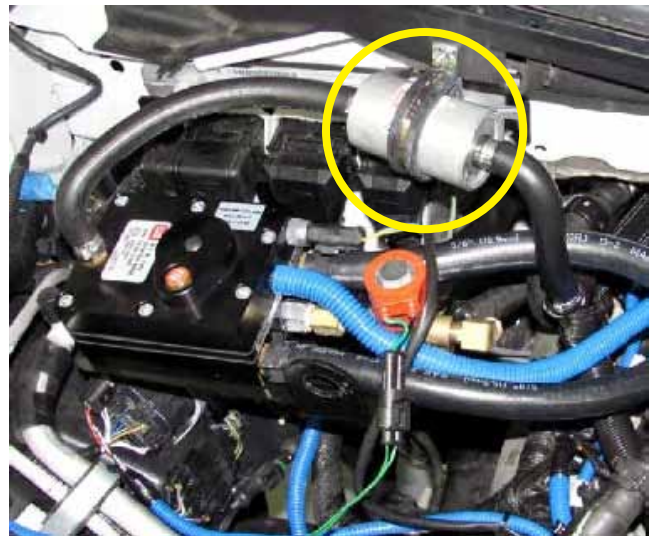
Figure 40. Secondary fuel filter, fuel feed hose installation
