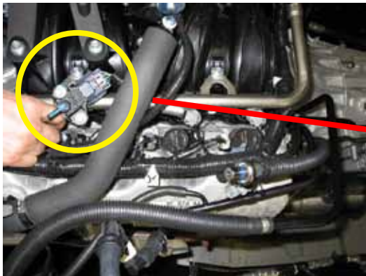
Figure 59. In a Roush CleanTech LPGI fuel system, the original gasoline injection pressure and temperature sensor (IPTS) connector is repinned for the propane fuel rail pressure and temperature sensor.
