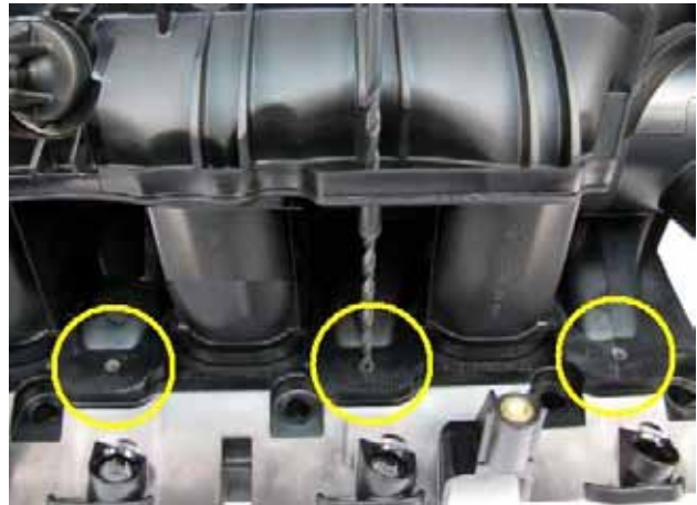
Figure 23. Drill locations for 2010 GM 6.0L engine
