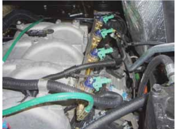
Figure 70. Completed CleanFUEL USA fuel-rail installation
