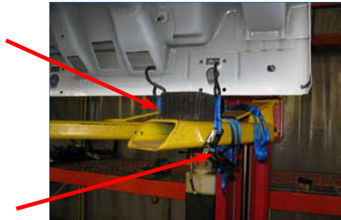
Figure 51. Preparing to separate the cab from the chassis
