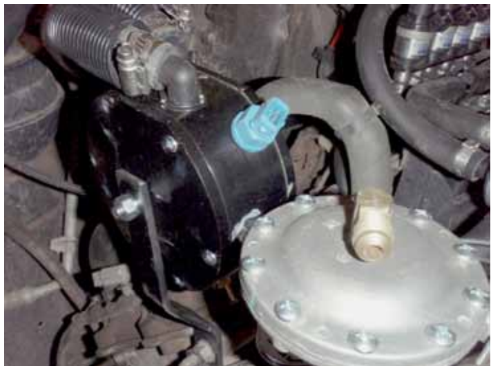
Figure 19. Vaporizer mounted directly on the engine
