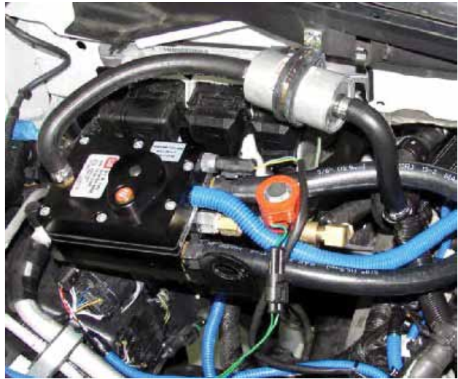
Figure 18. IMPCO Sequent vaporizer location on a 2010 Ford F-150
