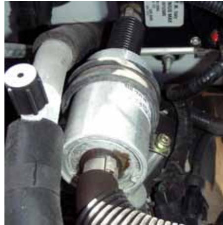
Figure 39. Secondary fuel filter, in-line installation
