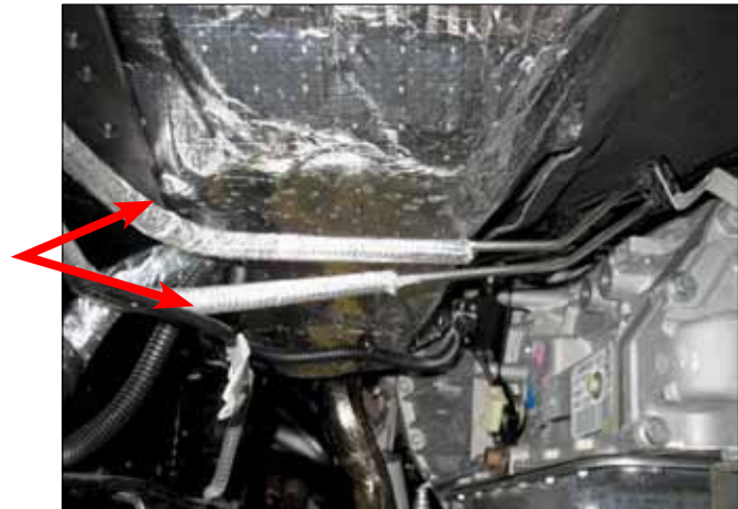
Figure 44. Routing of fuel supply and return lines
