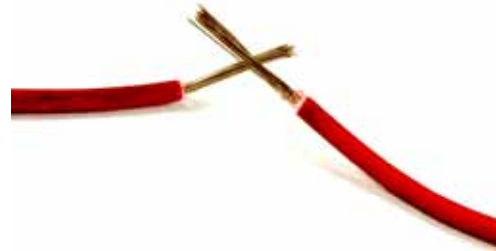
Figure 7. Twisting the wire connections together prior to soldering
