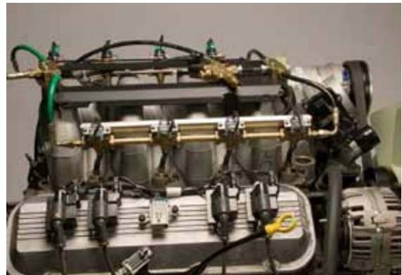
Figure 68. Completed CleanFUEL USA fuel-rail installation
