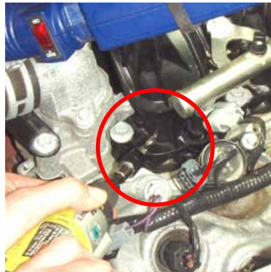
Figure 21. Drilling the manifold runner with a combination drill and tap bit
