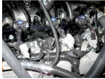
Figure 67. Completed Roush CleanTech fuel-rail installation
