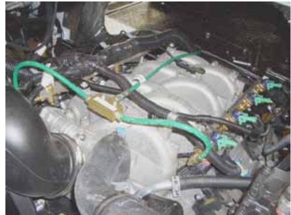
Figure 71. Completed CleanFUEL USA fuel-rail installation
