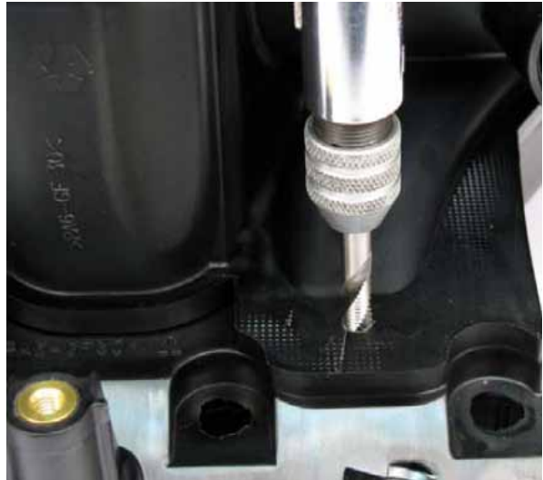
Figure 24. Drilling injector-nozzle holes for a 2010 GM 6.0L conversion
