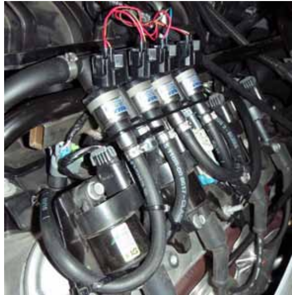
Figure 36. Fuel injectors mounted on ignition coil brackets
