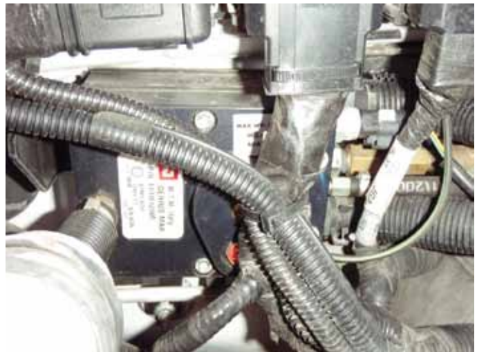
Figure 17. IMPCO Sequent vaporizer location on a 2008 or 2009 Ford F-150
