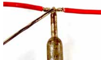
Figure 9. Proper method of heating a wire connection during soldering
