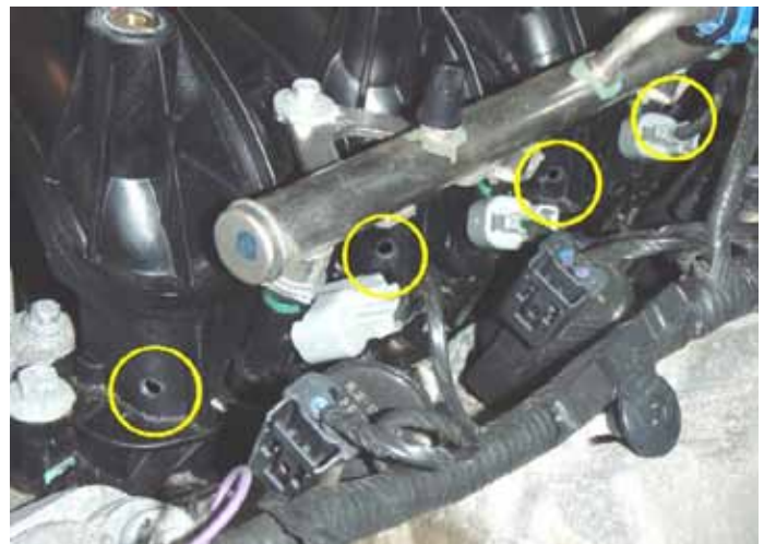
Figure 25. Drilled and tapped nozzle ports
