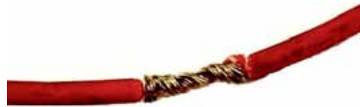
Figure 8. Mechanical connection prior to soldering
