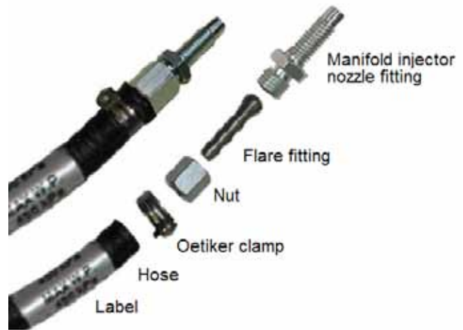
Figure 31. IMPCO injector hose end assembly
