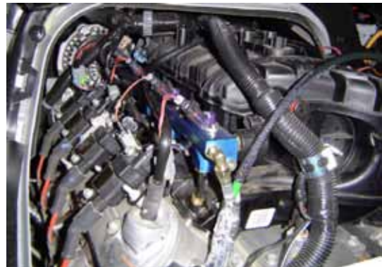
Figure 69. Completed CleanFUEL USA fuel-rail installation
