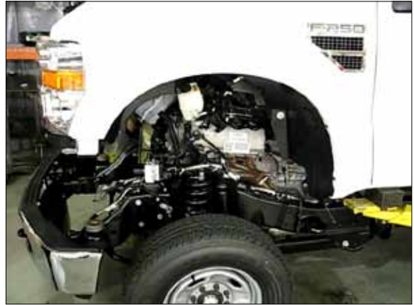
Figure 52. Lifting the cab from the chassis
