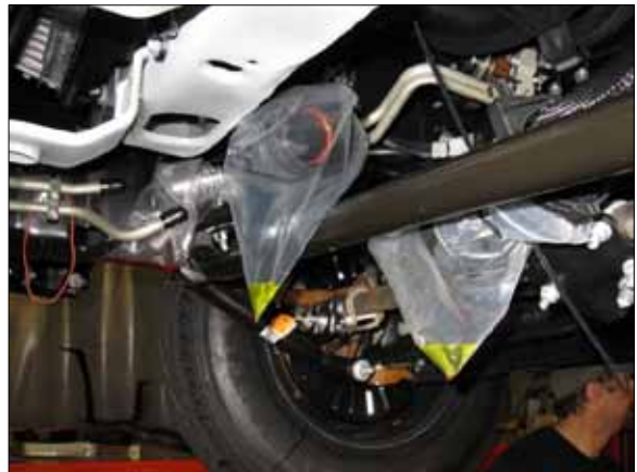
Figure 45. Radiator hose ends secured to prevent leaks
