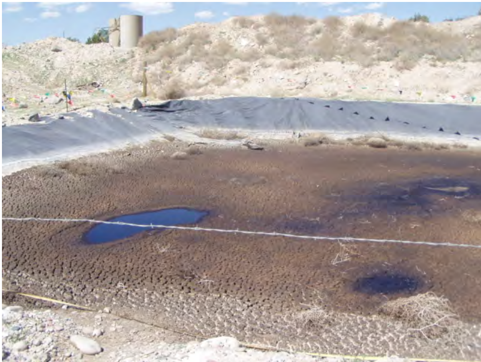
Figure 4. Reserve pit after fluids have evaporated. (USFWS Photo by P. Ramirez)
