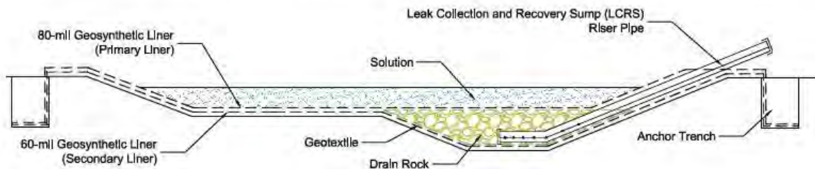
Figure 1: Process ponds are required to be double-lined with a functioning leak detection system.
