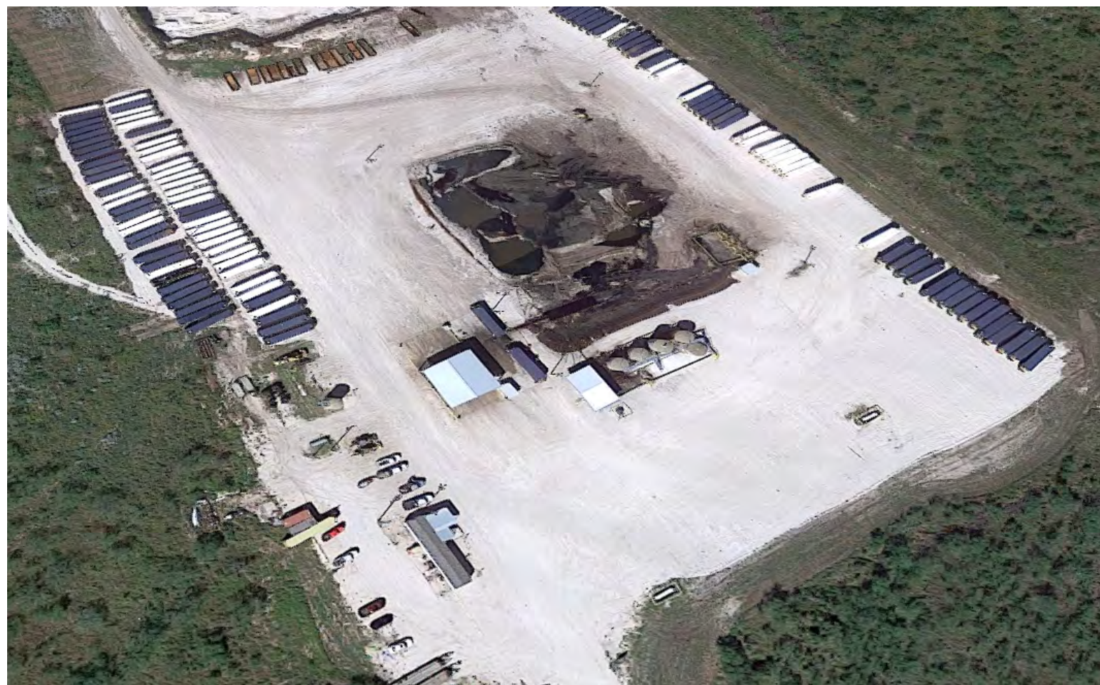
Built on a former caliche mine, the Blackhorn Environmental Services oil and gas waste disposal facility includes pits to separate solid and liquid material and other pits where waste is dried before being dumped in disposal cells. Credit: Google.
