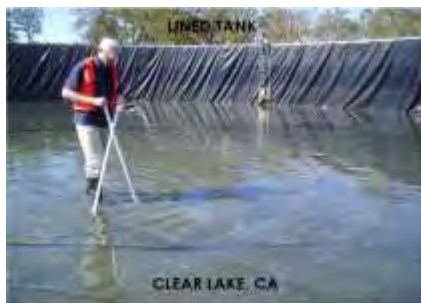
(b) Water covering geomembrane
