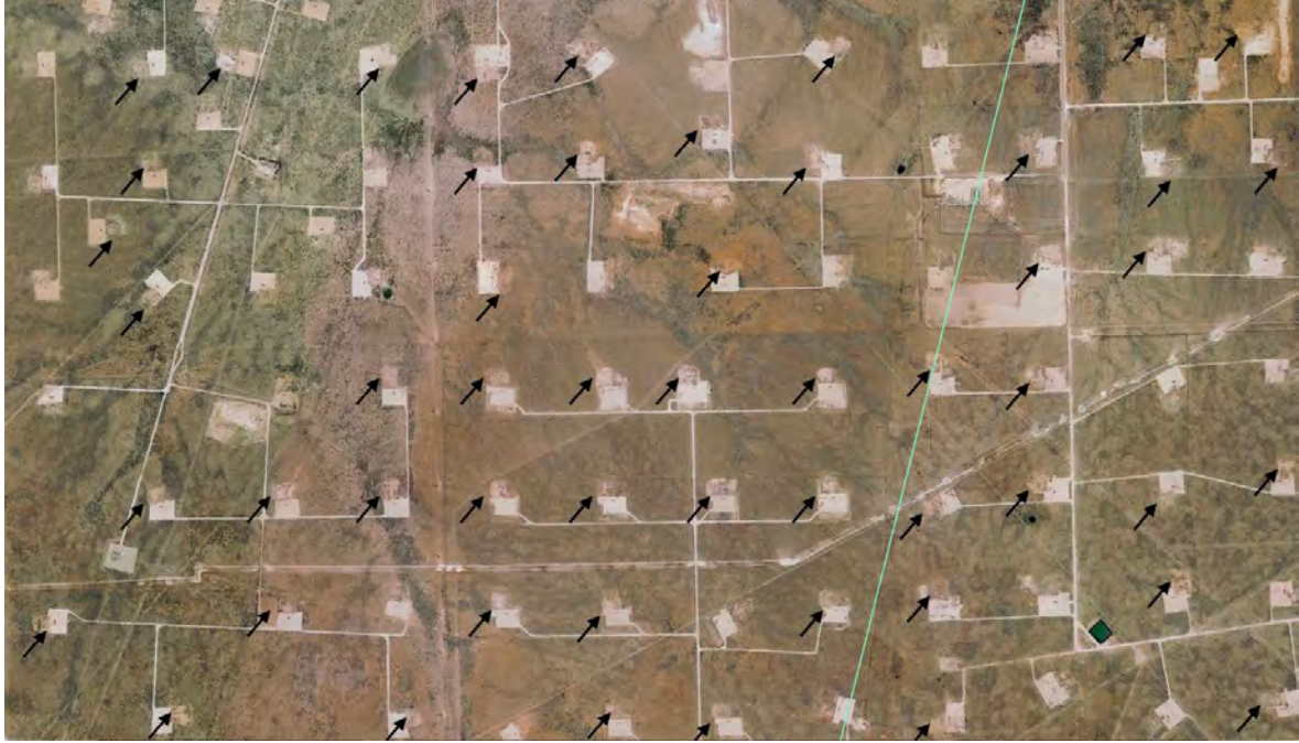
Figure 3. Permian Basin (Odessa) Drilling Density and Reserve Pits
