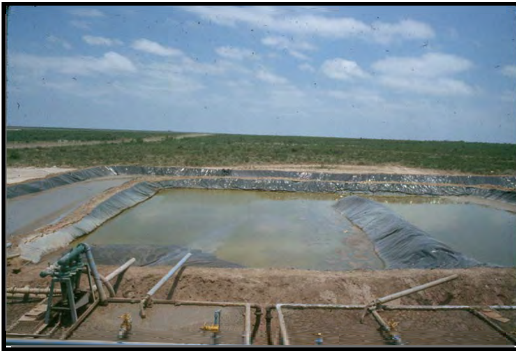
Photo 2. Oil well reserve pit containing drilling fluids.
