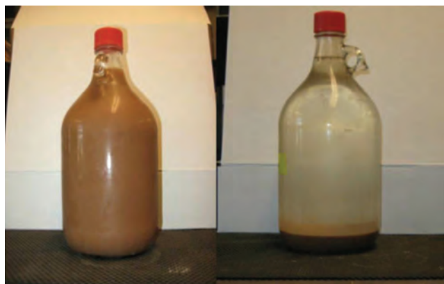
Figure 1. Example of water-base mud (WBM) pictured with (left) and without agitation.
